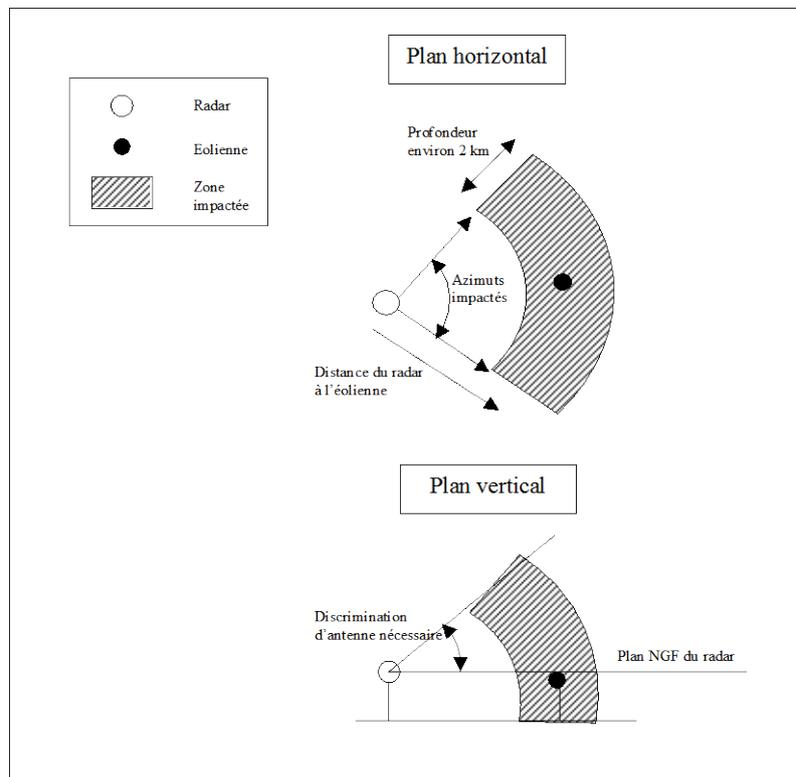
**Fig. 8:** Representation of the impact of a wind mill on Doppler mode
