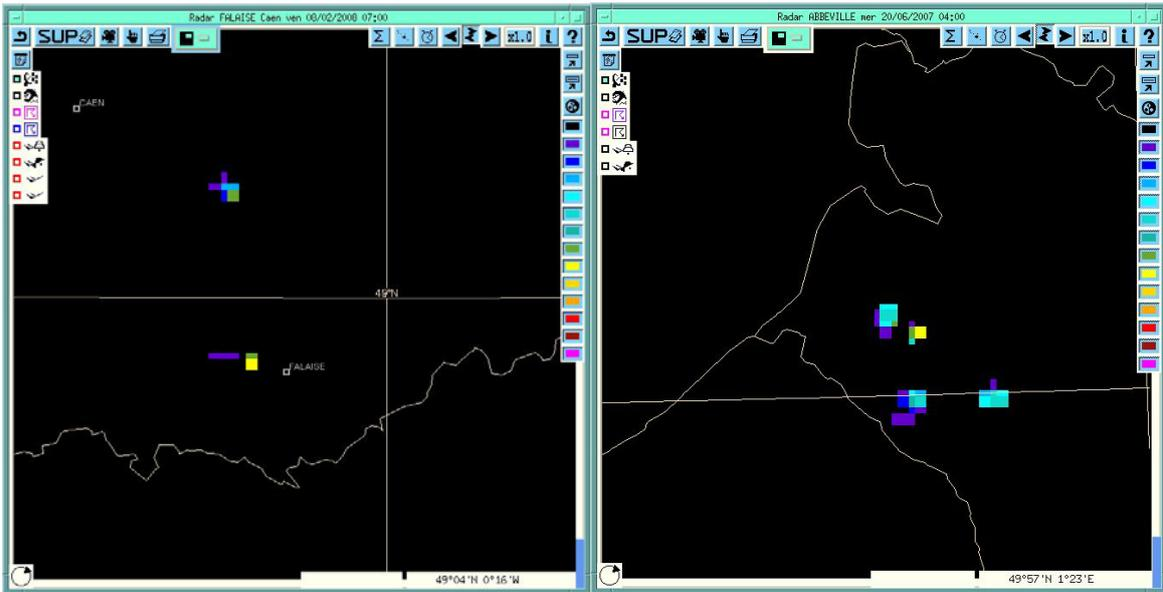
**Fig. 2:** Observation on 8 February 2008. Disturbance of precipitation data in vicinity of the French radar of Falaise. North, wind farm of Conteville at a distance of 19,9 km from the radar. South, wind farm of Aubigny Soulangy at a distance of 3.5 km from the radar.
