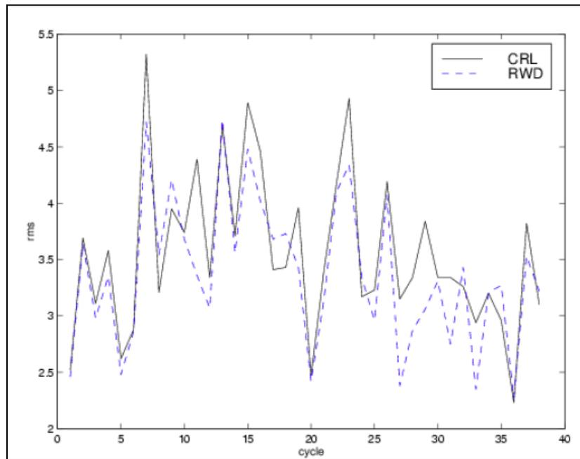
**Fig. 13:** RMS forecast verification scores for 700 hPa wind speed, verified against radiosonde data, from experiment with (RWD) and without (CRL) radar radial wind super-observations. The data period is 1 – 10 December 1999.
