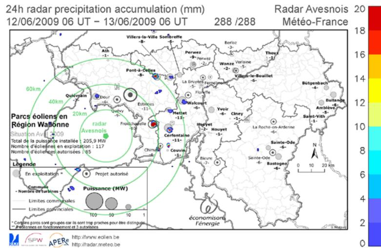
**Fig. 6:** Superposition of a 24h radar precipitation accumulation for the Avesnois radar (in [mm], scale on the right) with the location of the wind farms indicated by circles. The selected day is a day without precipitation (12 June 2009 0600 UTC – 13 June 2009 0600 UTC). Image kindly provided by M. Reyniers (RMI).
