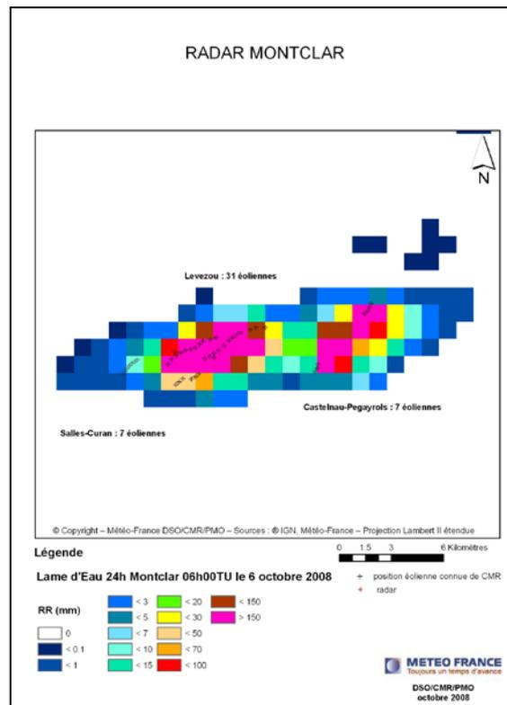
**Fig. 4:** Wind farms in Salles-Curan, Castelnau-Pegayrols and Lévezou located between 19 and 31 km from the French radar of Montclar produce an impact zone on precipitation accumulation data extending 25 km long and 5 km width. It renders data unavailable over an area of about 125 km<sup>2</sup>.
