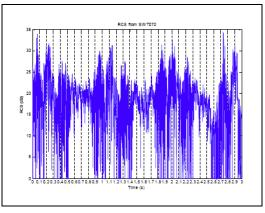
Fig. 1.a: Time variation (3s) of 3 GHz RCS of an Enercon E66 wind mill for a 39° rotor orientation (QuinetiQ, 2003).
