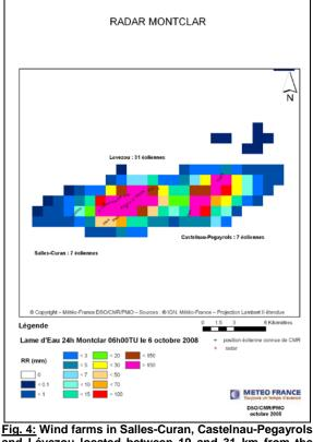
Fig. 4: Wind farms in Salles-Curan, Castelnau-Pegayrois and Lévezou located between 19 and 31 km from the French radar of Montclar produce an impact zone on precipitation accumulation data extending 25 km long and 5 km width. It renders data unavailable over an area of about 125 km<sup>2</sup>.
