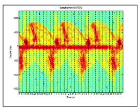
Fig. 1.b: Time variation (3s) of the Doppler spectrum of an Enercon E66 wind mill for a 39° rotor orientation (QuinetiQ, 2003).
