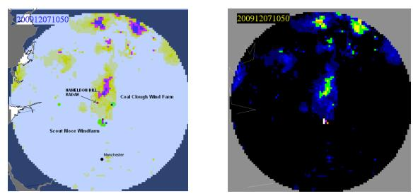
Fig. 7: Wind turbine clutter in the precipitation (left) and reflectivity imagery (right) for the Hameldon Hill radar (UK) on 7 December 2009 1050 UTC. The resolution is 1 km. Images kindly provided by S. Holton (UKMO).
